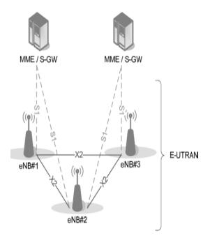
Figure 3: LTE (release 8) architecture
