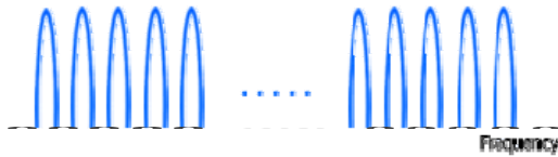
Fig2. Frequency Division Multiplexing
