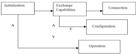
Fig.2 State machine for Wireless network control protocol
