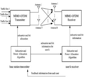
Fig.2. Block diagram of multiple antenna OFDM multicast system.
