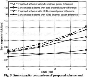
conventional one in multicast system when the SNR is low.
