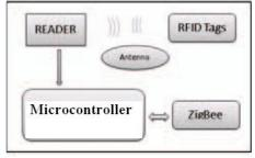
Fig. 1 : Sensor node schematic of RFID&ZigBee
