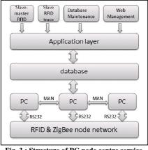
Fig. 3 : Structure of PC node centre service
