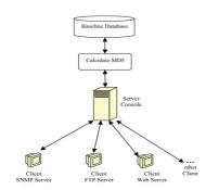
Fig. 7 : System architecture of MD5
