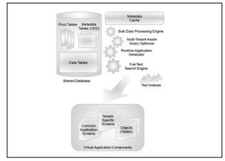
Fig. 1 : Force.com Platform Architecture.
