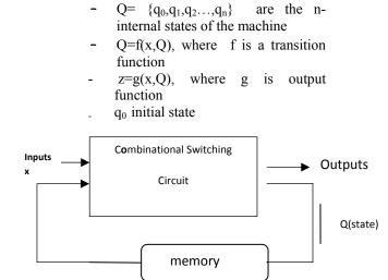
Fig. 1.1 Sequential Switching Circuit
