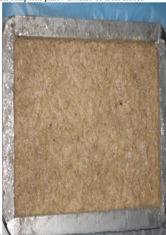
Fig6.1 composite plate fabrication
