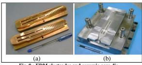
Fig. 8 : EDM electrodes and ceramic core die
