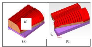
Fig. 12 : CAD models of electrode design for (a) Split line and (b) cavity for concave die block
