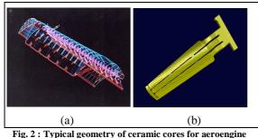
turbine (a) blade and (b) vane
