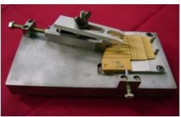
Fig. 15 : Core finishing fixture
