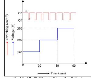
Fig. 5 Test Profile (Time vs. Voltage & switching)
