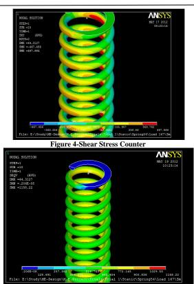
Figure 5-Eq. Von Mises Stress Counter
