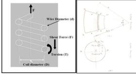
Figure 1- Elemental Section of Helical Coil Compression Spring [1]
