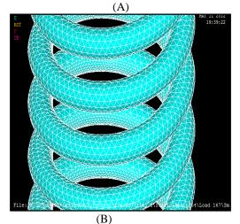
Figure 2- Solid Model (A) and FEM Model (B) with Tet Mesh (SOLID 187)
