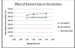
Figure 3- Comparison of Different Meshing Types
