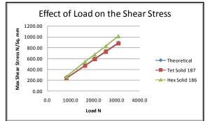
Figure 5-Load Vs Shear Stress Effect on spring
