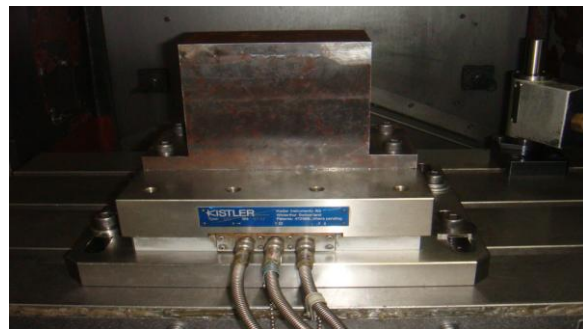
Fig. 6. Workpiece clamped to dynamometer fixture
