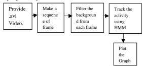
Figure 1. Shows the block diagram for human activity recognition.
