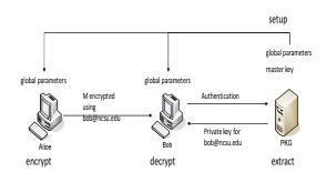
Fig 2 : Framework of ID-based encryption
