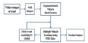
Fig.1: Flow chart for Multiple Vehicle Tracker
