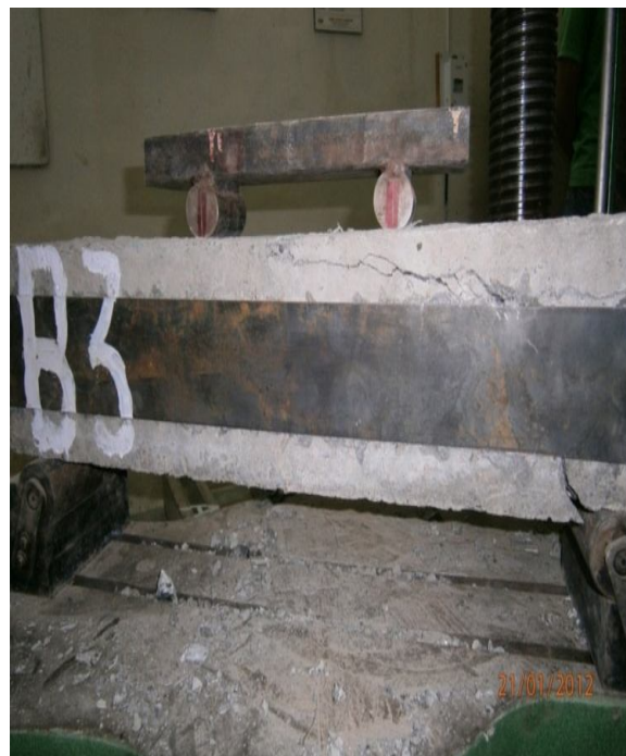
Figure 4 Typical failure of reinforced concrete beam strengthened with continuous steel plate
