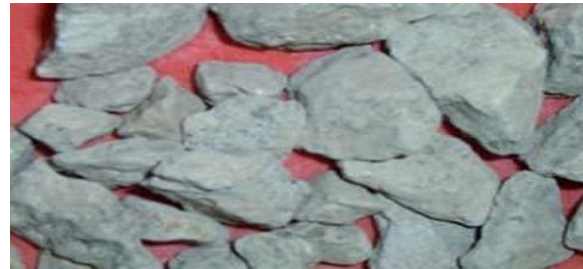
Figure 1 Coarse aggregate segregated from concrete waste
