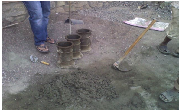
Figure 9 Filling of Concrete Mix in Cylinders
