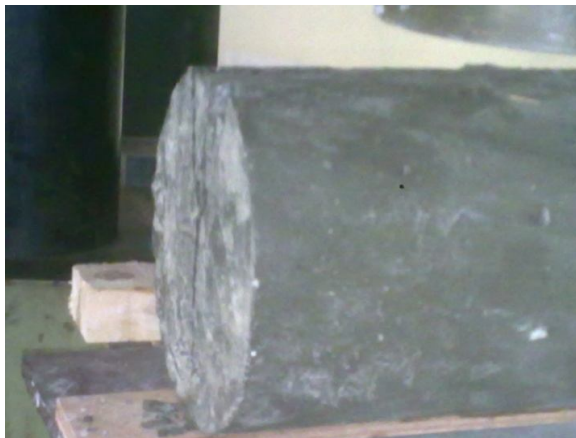
Figure 13 Concrete Cylinder specimen before failure
