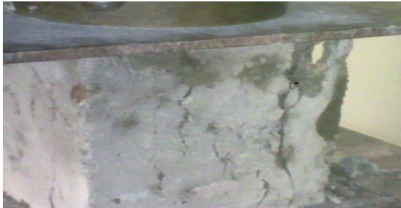
Figure 12 Concrete cube specimen after failure
