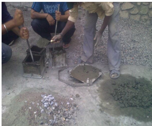
Figure 8 Filling of Concrete Mix in Cubes
