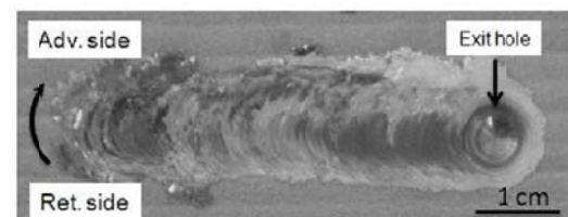
Fig. 6. The photo of the FSS surface of Zn-Y 2 O 3 -ZrO 2 cold sprayed coating
