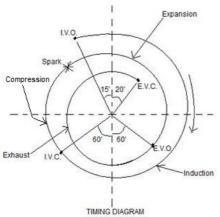
Fig. 2: Timing Diagram of a Petrol Engine
