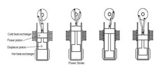
Fig. 4: Working of a Stirling Engine
