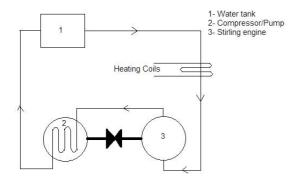
Fig. 8: Layout of Closed Water Cycle
