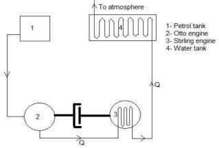
Fig. 7: Layout of Open Petrol Cycle
