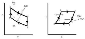
Fig. 5: Stirling Cycle
