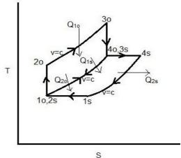
Fig. 9: T-S diagram of Dual Cycle
