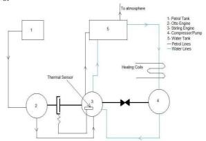
Fig. 6: Working Layout of Concept ECO-TWINGINE
