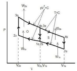
Fig. 10: p-V diagram of Dual Cycle
