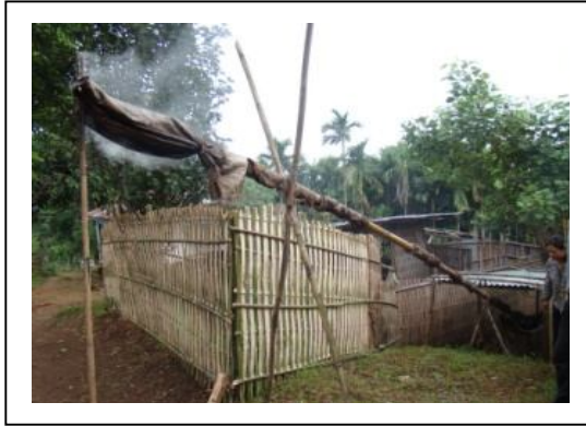
Fig. 3 : Hollow Bamboo Shaft covered with moist jute packing used as condenser for producing bamboo vinegar
