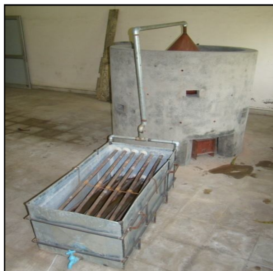
Fig. 7 : Setup of Condenser at IITG by fitting to developed furnace
