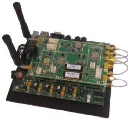
Fig: SFF SDR Development Platform
