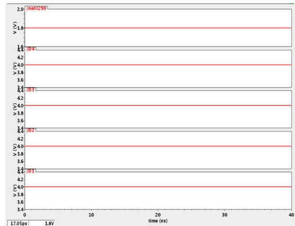
Fig.10: Transient response for V_{in} = 1.8V , output will be 1111
