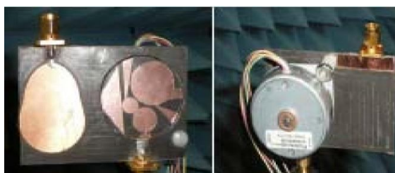
Fig. 5- The fabricated prototype combined with a UWB sensing antenna and a frequency reconfigurable communicating antenna. [8]
