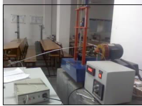
Fig.7: Experimental setup to study fixed wing dynamics.
