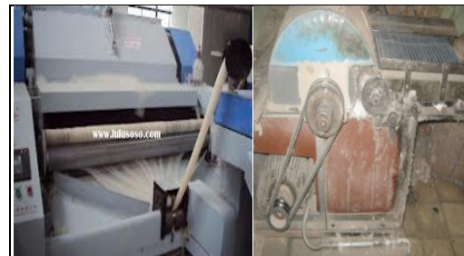
Fig. - Carding Machine use in Textile Industry and Pinjanalaya Carding Machin
