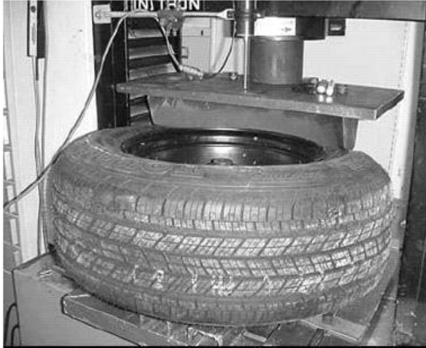
Figure 1. Bead unseating test
