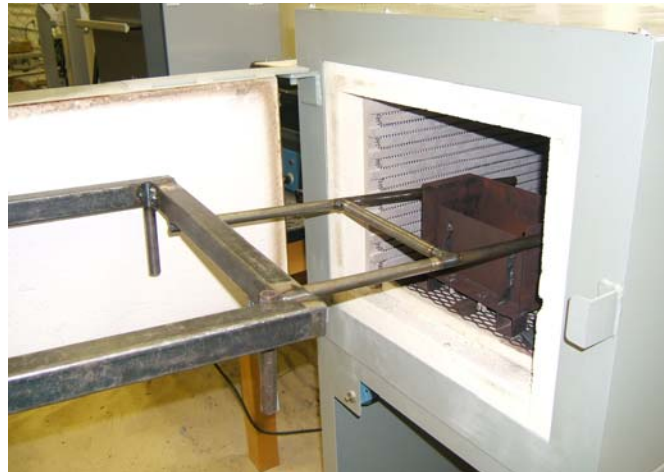
Figure 3.14 - Mold Carrier Removal Process (staged)
