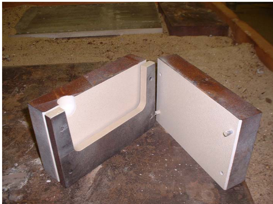
Figure 3.2 - Three-piece Steel Mold (partially assembled)
