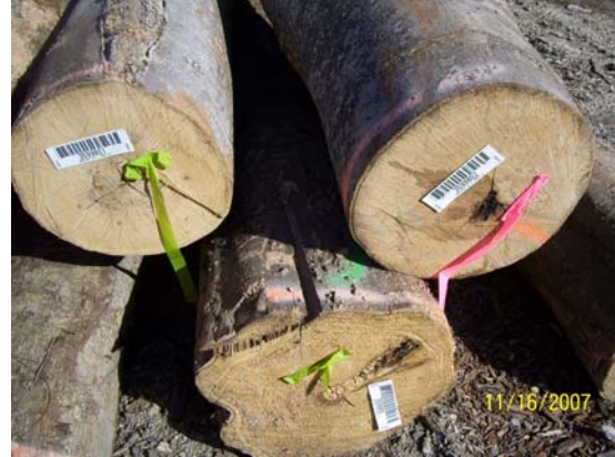
B. 2-Month Check-up; Notice Relatively no Checks/Splits & Minimal Surface Discoloration.
