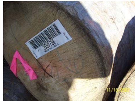
B. Control Log Illustrating Discolorations Roughly 1 Month After Segregated.
