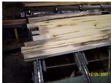
B. Y (1-6) 4.0% SB + Anchorseal Heavy Discolorations
