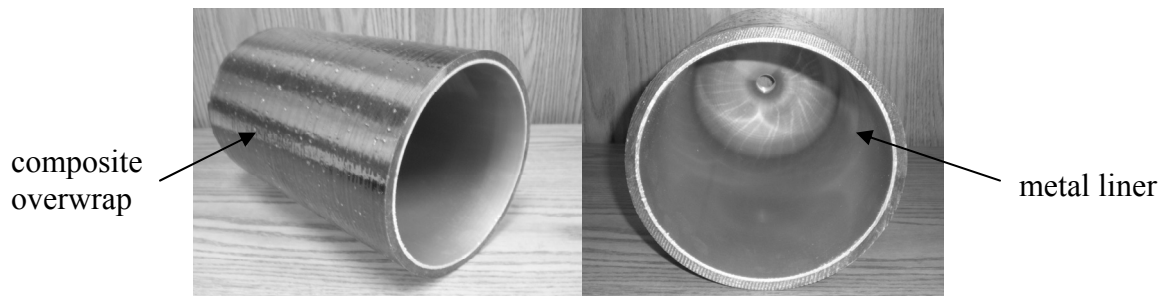
Figure 2.1: Cut-away picture of a COPV. Metal liner may be treated to either promote or prevent adhesion to overwrap.
