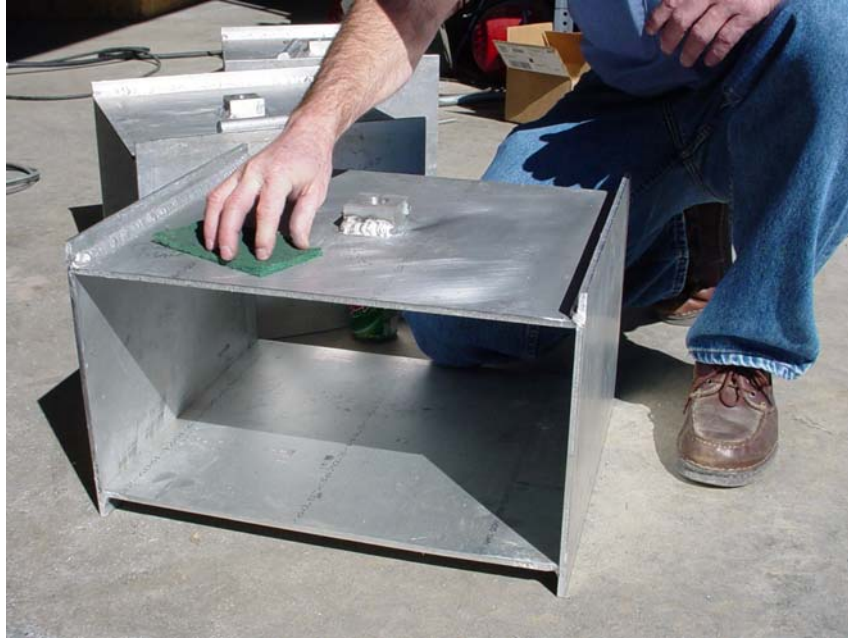
Figure 3.49 Partially Assembled Filter Cavity
