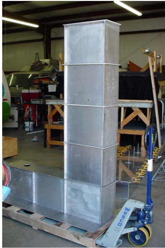
Figure 3.54 Folded Waveguide Rear during Assembly
