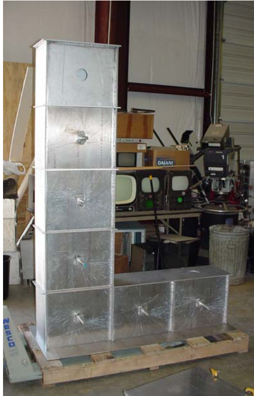
Figure 3.53 Folded Waveguide Filter Front during Assembly
