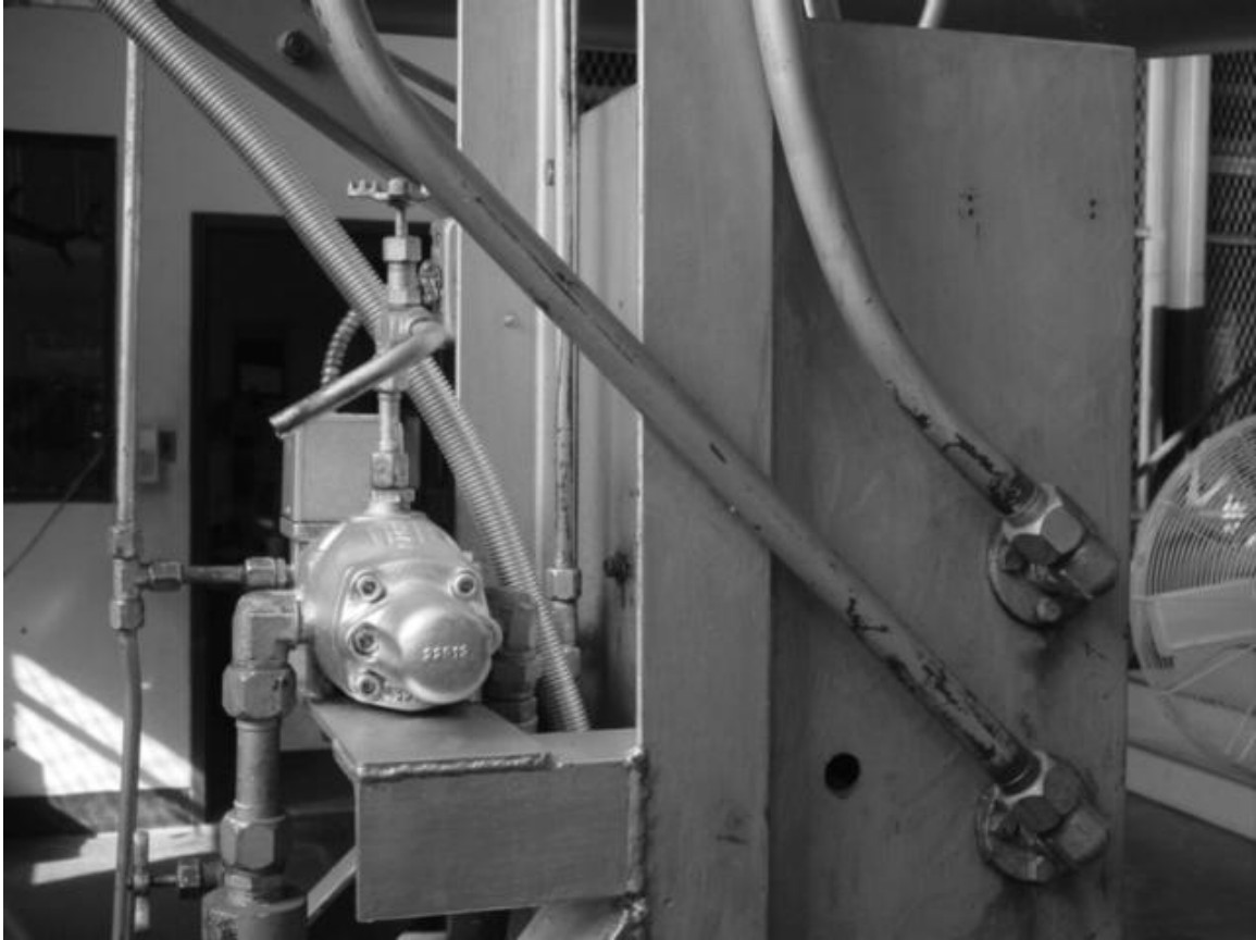
Figure 4 Speed-Restriction Valve and Servovalve
