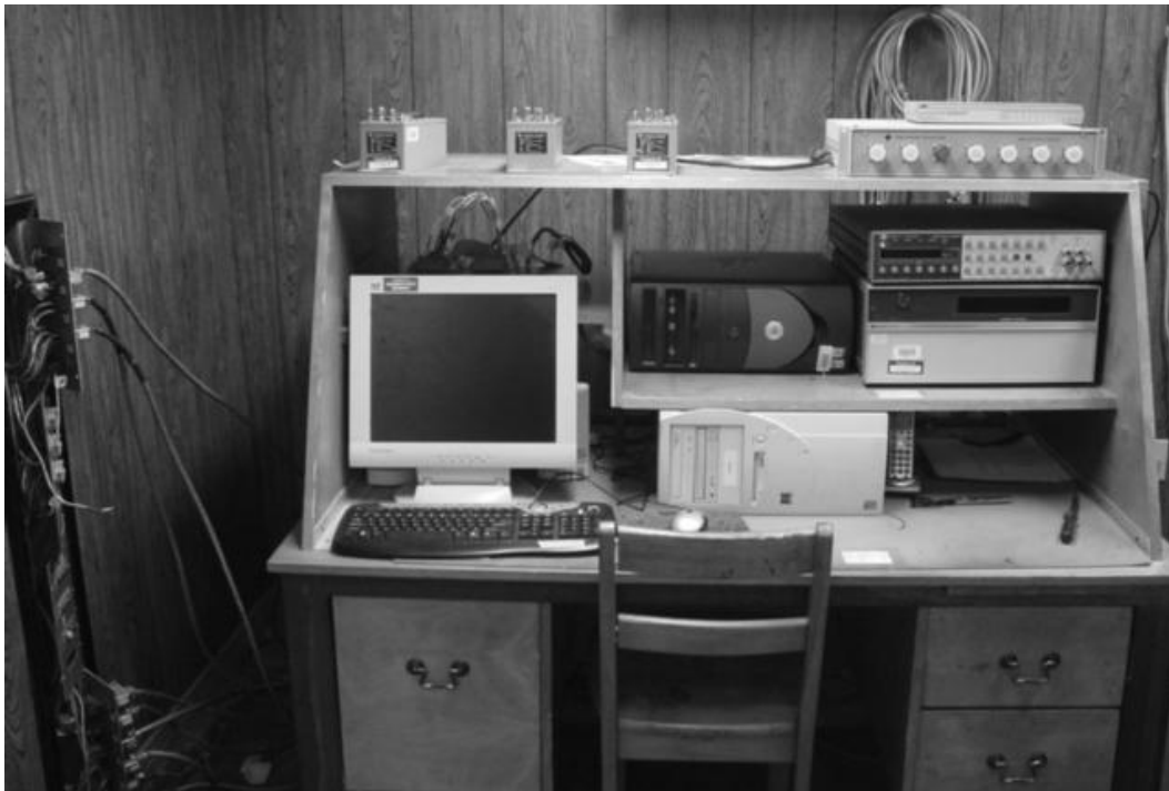
Figure 6 WTCR Showing Connection slot, HP 3495A Scanner, and Netscanner
