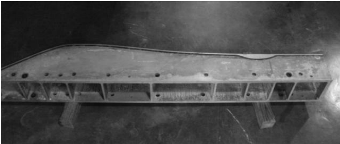
Figure 11 Nozzle Block Showing the Internal Structure
