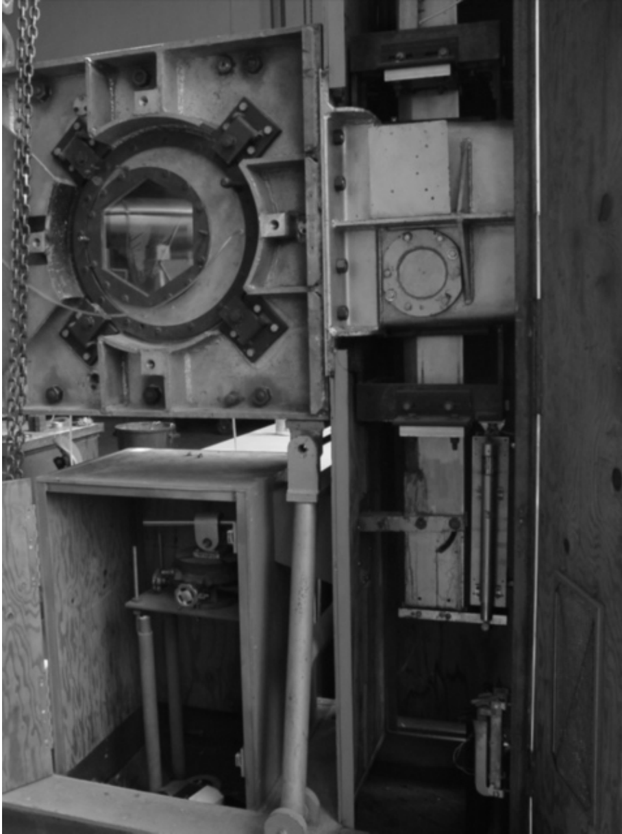
Figure C.8 Sting System for Tunnel
