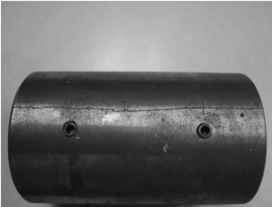
Figure C.7 Cracked Collar for Inlet Butterfly Valve
