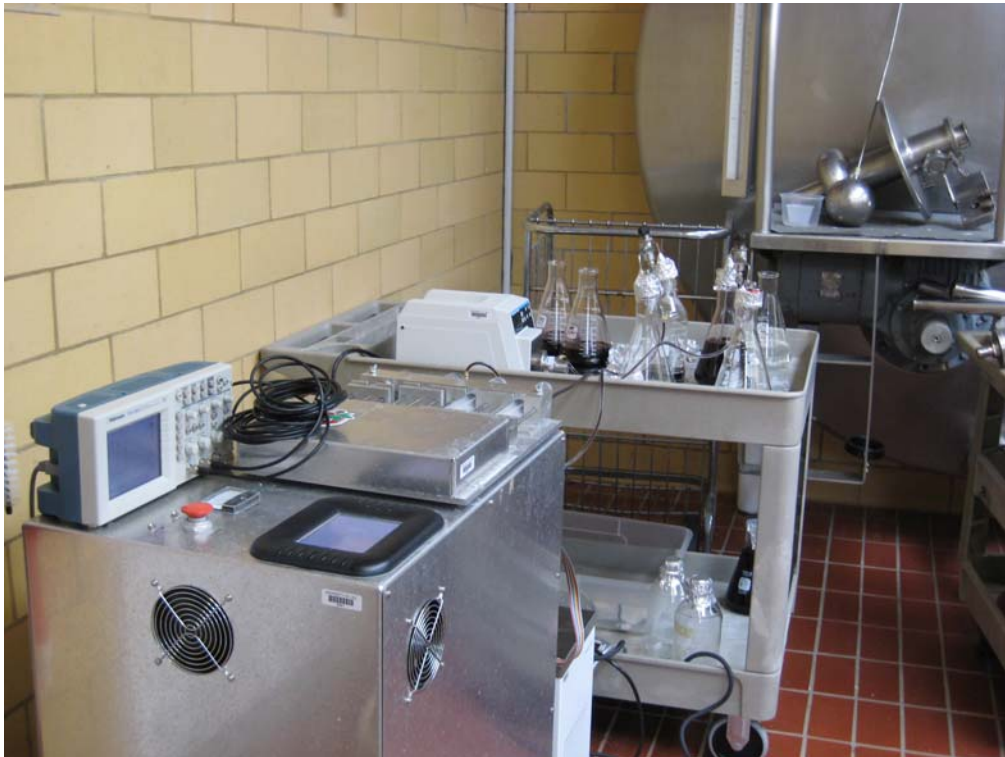
Figure 8. OSU-4K Pulsed Electric Field Equipment.
