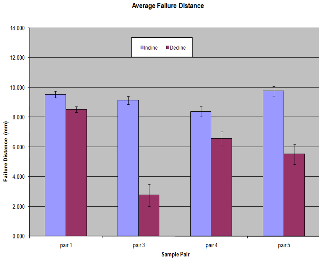
Figure 4.12. Graph of comparison of average failure forces in implant designs in testing on an incline and on a decline.
