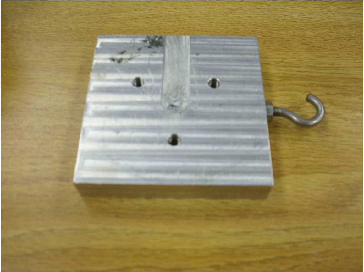
Figure 4.2. Picture of top fixation device used in setup for testing in shear.
