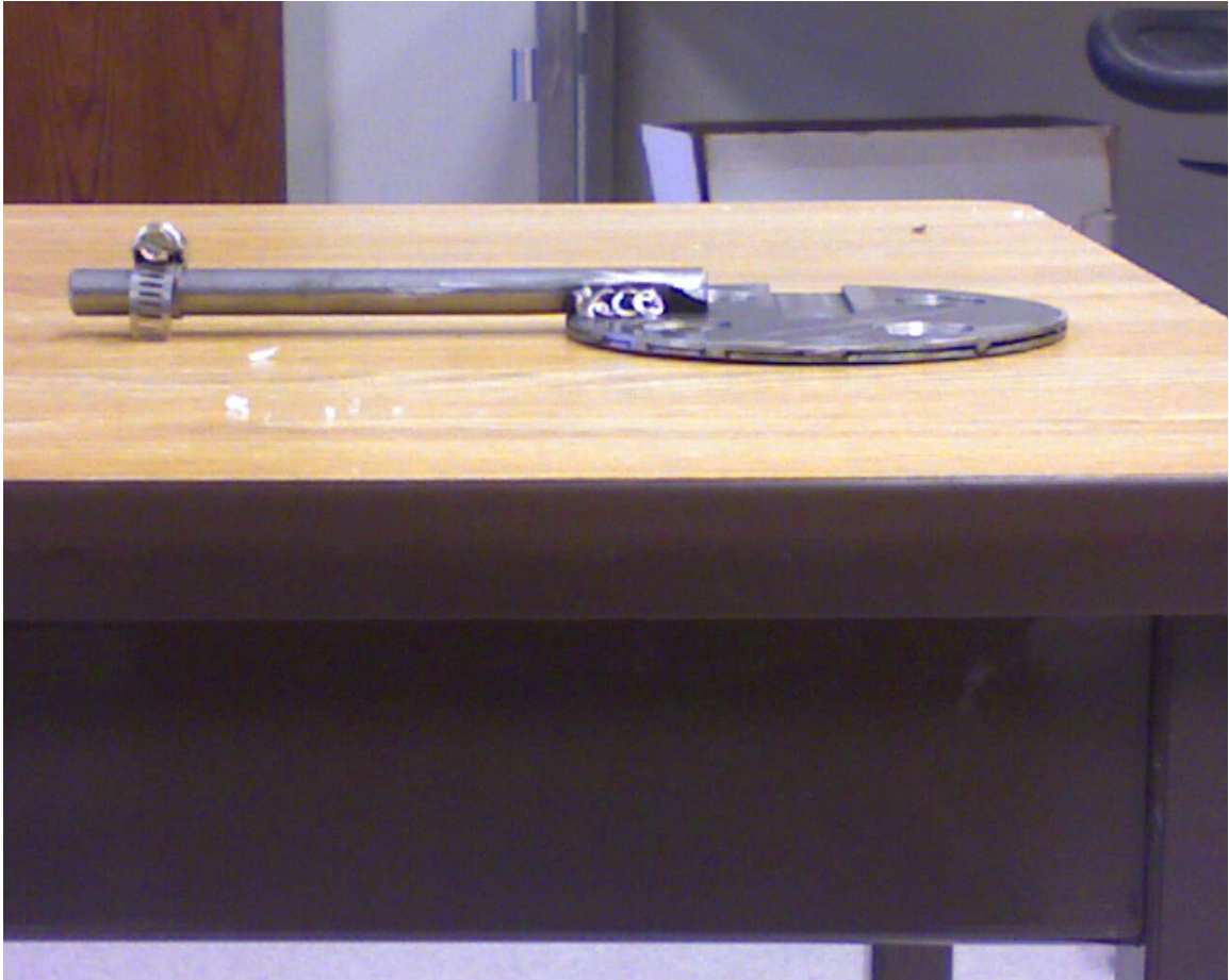
Figure 5.5. Modified bottom fixation device for torsional testing with a load cell
