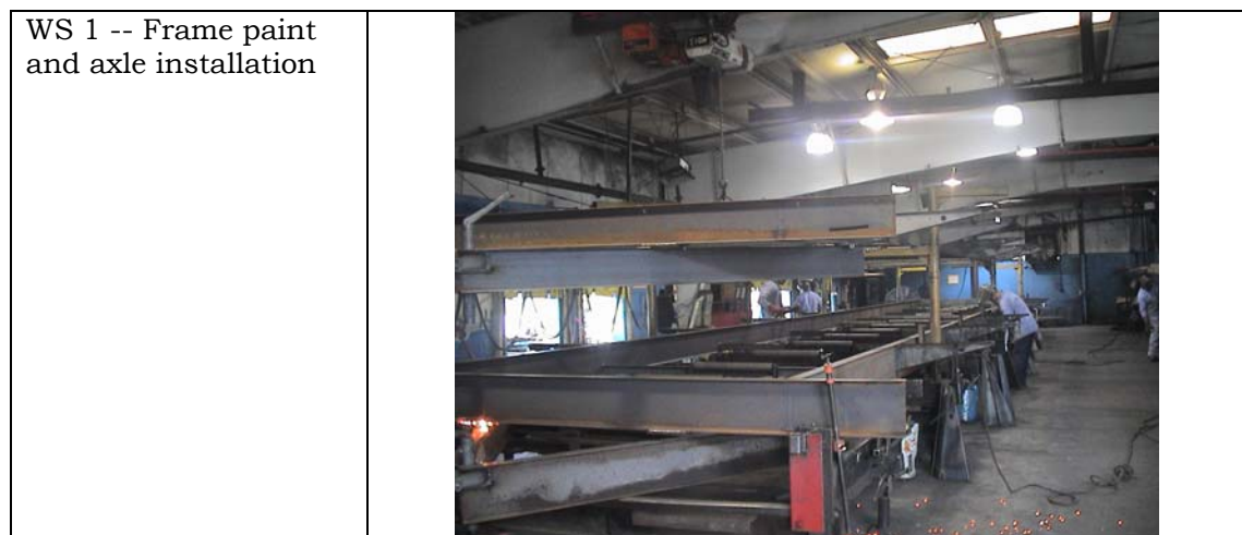
Figure B.3 The assembly line station breakdown in the Buccaneer Homes
