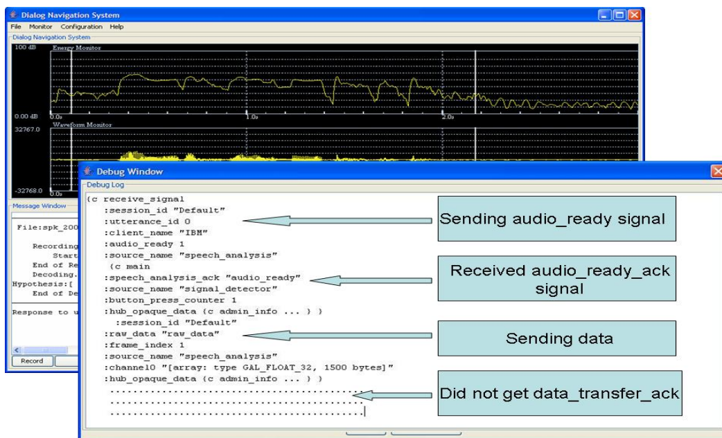
Figure 20 A debug window showing an audio data transfer error.
