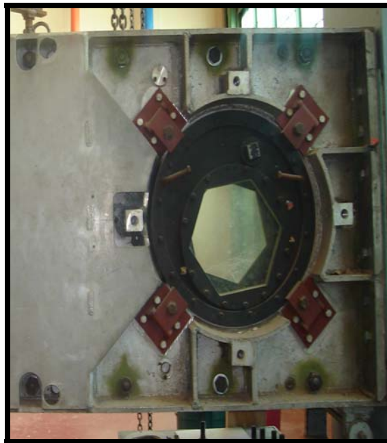
Figure 2.3 Supersonic Wind Tunnel Test Section Access and Viewing Port.
