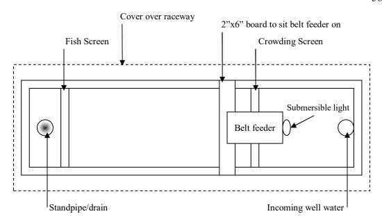
Figure 3.1 Design of raceway used to feed-train pond-reared walleye fingerlings (Top view).
