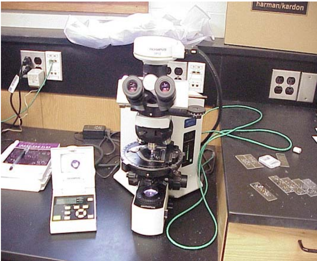
Figure 7: Polarized Light Microscope (PLM) with a DP12 camera at the top
