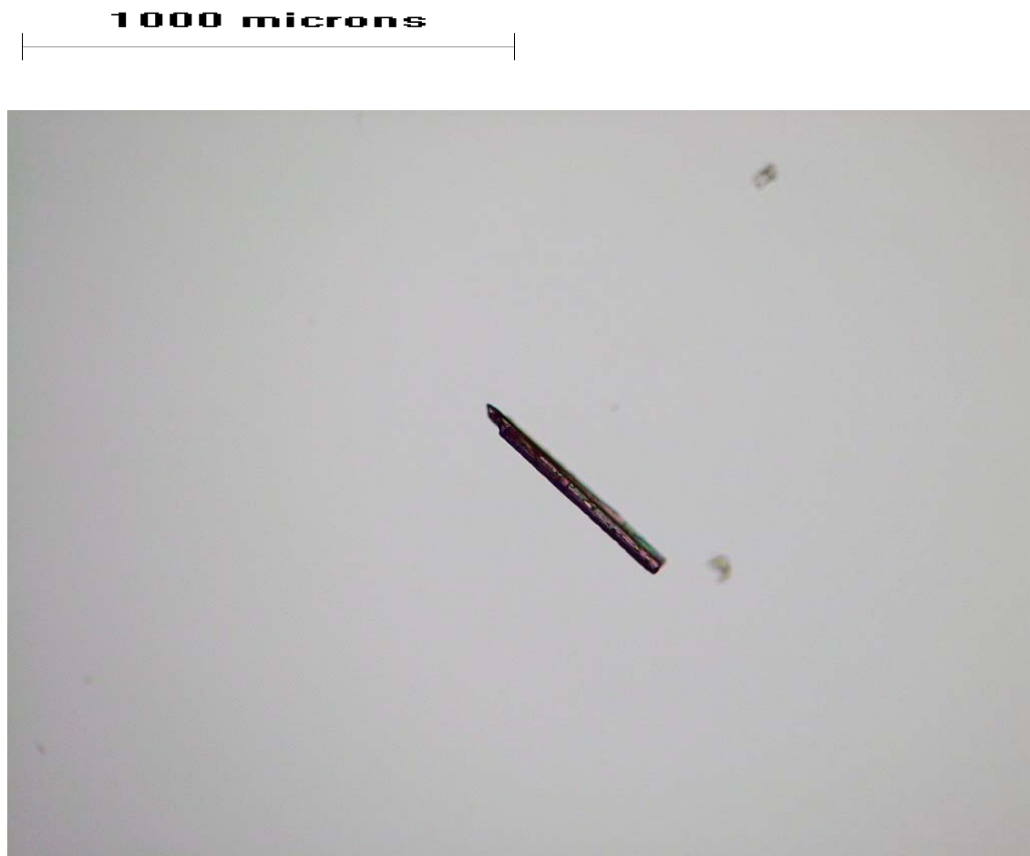
Figure 10: The image of a broken urea crystal caused primarily due to excess growth rate
