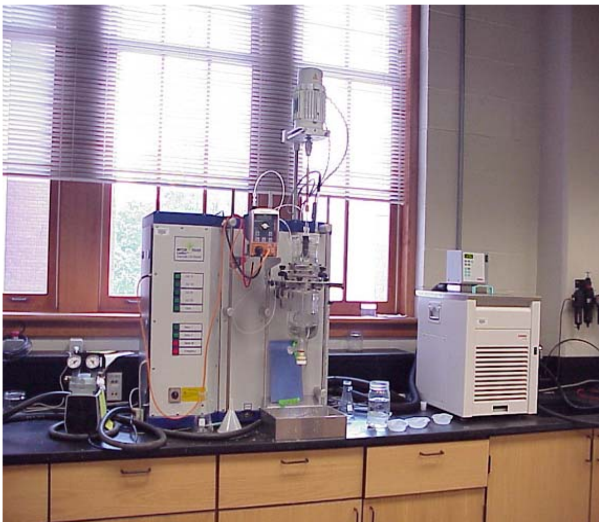
Figure 4: The Mettler Toledo LabMax (automated laboratory reactor) with the Chiller to its side
