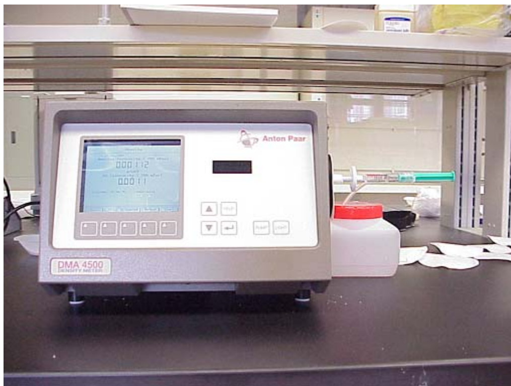
Figure 5: Anton Parr density meter with a syringe in the side that feeds the sample in to it.
