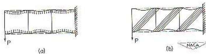
Figure 5.- Secondary actions in diagonal-tension beams .
