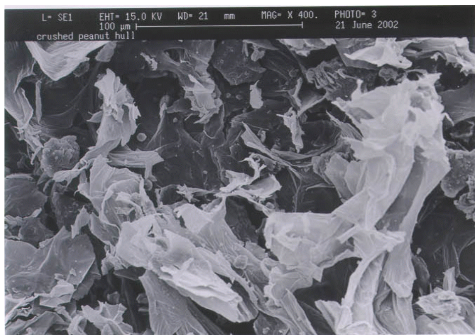
Figure F.12. SEM micrograph of crushed peanut hulls. Magnification: 1 x 400.
