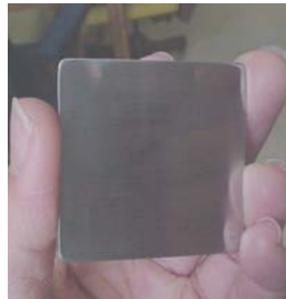
Figure 1. A polished Co-Cr-Mo alloy plate used for corrosion tests. It was wet polished using SiC sandpaper up to 1200 grit, cleaned and passivated according to ASTM F86 to simulate clinical implant surface preparation.
