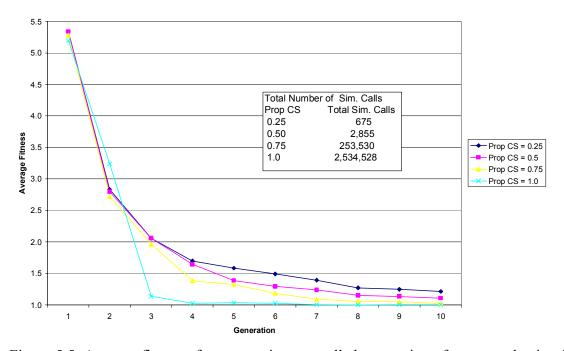
Average Fitness using controlled proportion of CS for Test function-1
