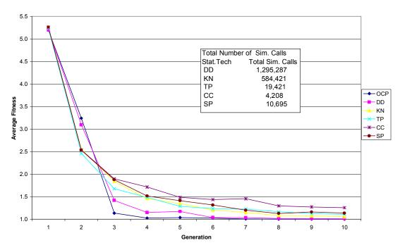
Figure 5.7 Average Fitness of parents for modified selection mechanisms at  $\alpha$ =0.1 for Test function-1
