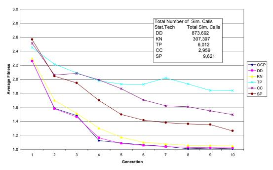
Figure 5.16 Average Fitness of the solutions for modified selection mechanism at  $\alpha = 0.4$  for Test function-2
