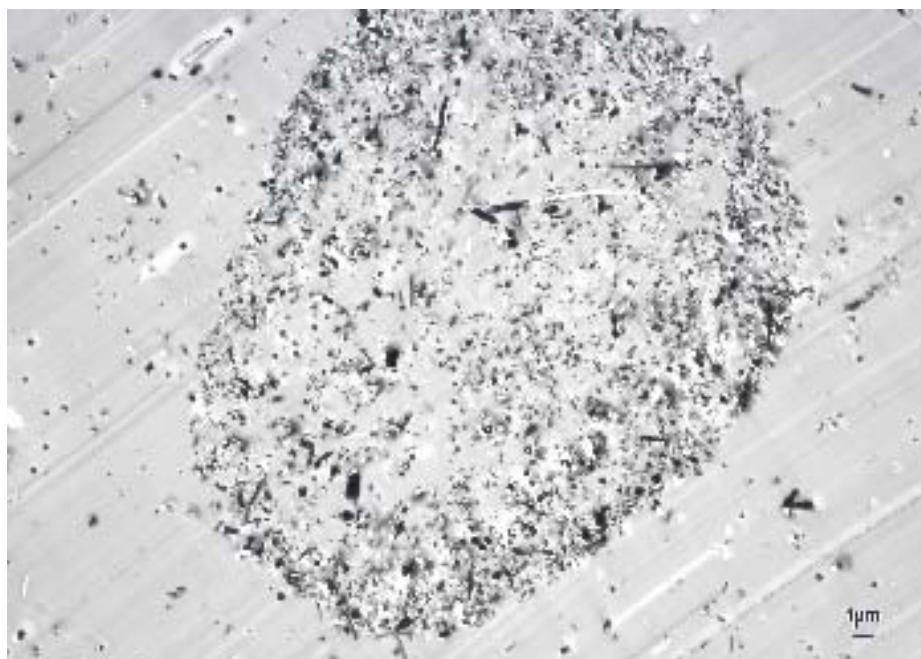
Figure 3.52 Unoxidized VGCF/Epoxy resin composite. A nest region with high concentration is present in matrix with a surrounding region of lower fiber density. Magnification is 2000X.
