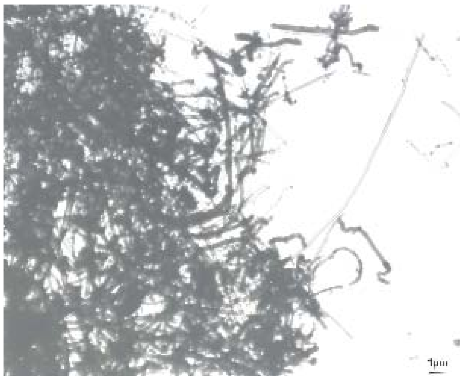
Figure 3.50 A clump of unoxidized VGCFs. Magnification is 2000X.
