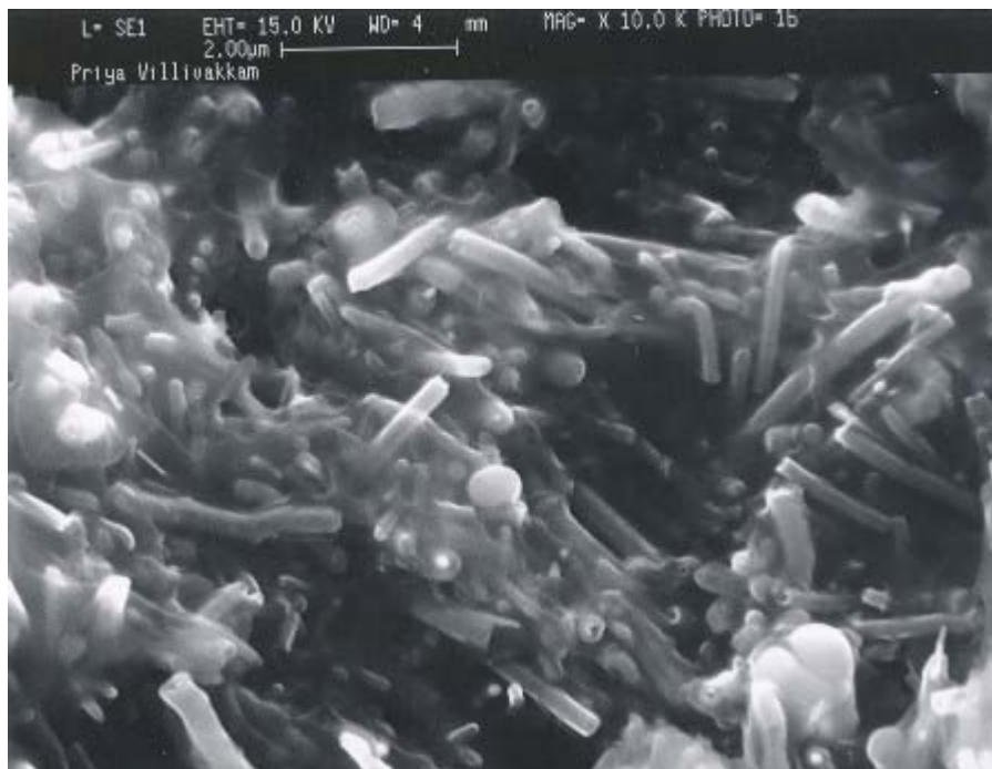
Figure 3.44 The fractured end on unoxidized VGCF/Epoxy resin composite at a magnification of 10K.
