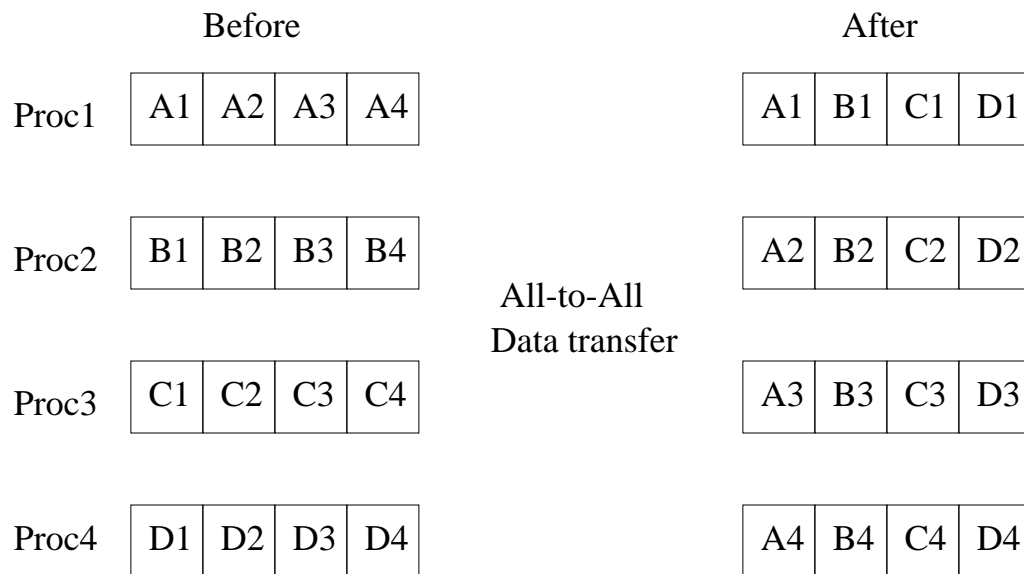
Figure 4.1 Data movement in an all-to-all communication
