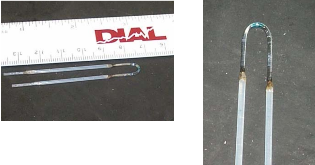
Figure 4.3: The implemented U-shaped (bent) Probe Sensor
