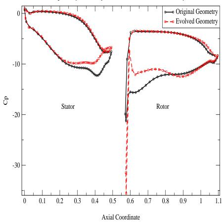
Figure 4.8:  $C_p$  Comparison of DAT with Increased Combination of Average  $C_x + C_y - |C_d|.$
