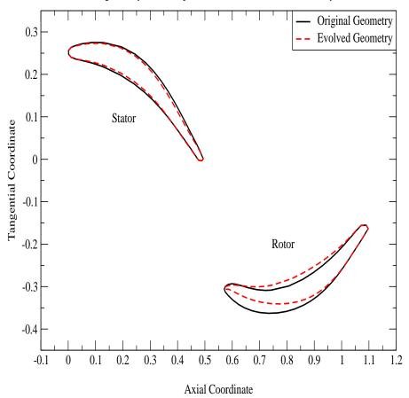
Figure 4.7: Geometry Comparison of DAT with Increased Combination of Average  $C_x + C_y - |C_d|$ .
