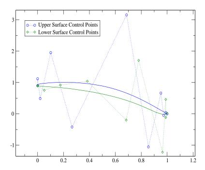
Figure 3.1: Approximated Geometry with Bezier Points Overlaid
