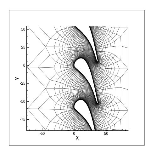
Figure 4.9: Original VKI Geometry and Structured Grid
