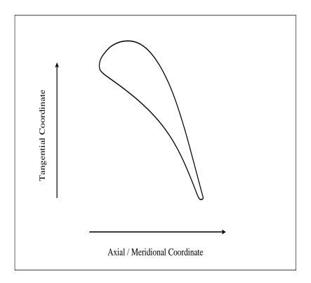
Figure 3.5: Coordinate system used in flow solver
