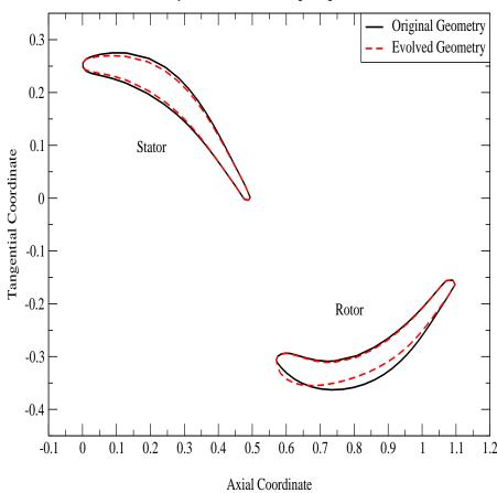
Figure 4.3: Geometry Comparison of DAT with Increased Average  $C_y$ .
