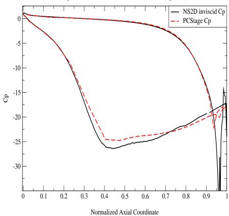
Figure 4.17:  $C_p$  Comparison for VKI with Increased Combination of  $C_x + C_y - |C_d|$ .
