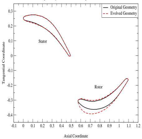
Figure 4.1: Geometry Comparison of DAT with Increased Average  $\mathcal{C}_x$  .
