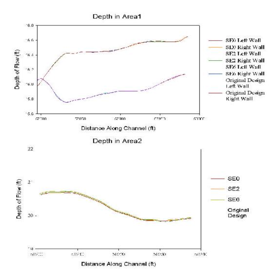
Figure 4.10: Depth Profile in Area1 and Area2 for Super Elevation Test Cases.
