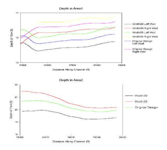
Figure 4.15: Water Depth Profiles in Area1 and Area2 for Width Test Cases.
