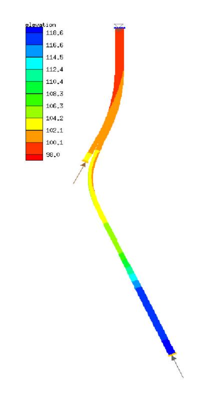
Figure 4.27: Layout and Bed Elevations of the Improved Design.
