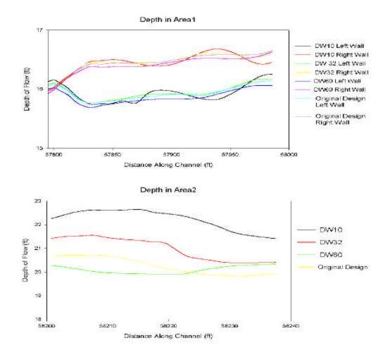
Figure 4.17: Water Depth Profiles in Area1 and Area2 for Divider Wall Test Cases.
