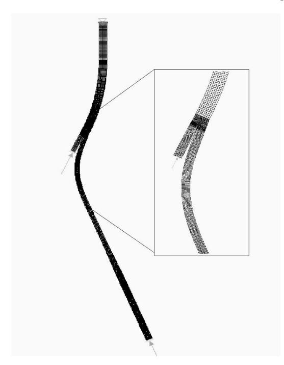
Figure 4.31: Initial Grid for the Radius of Curvature Problem.
