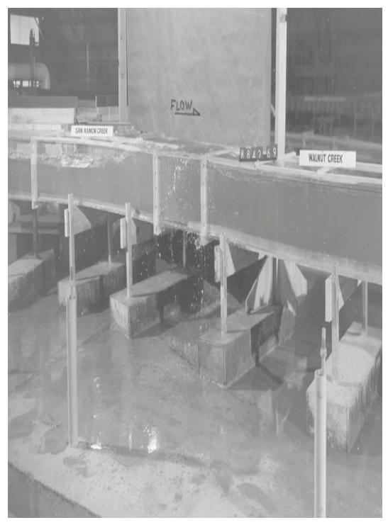
Figure 2.7: Depths Exceeding Wall Heights Downstream of Junction [Davis 87].
