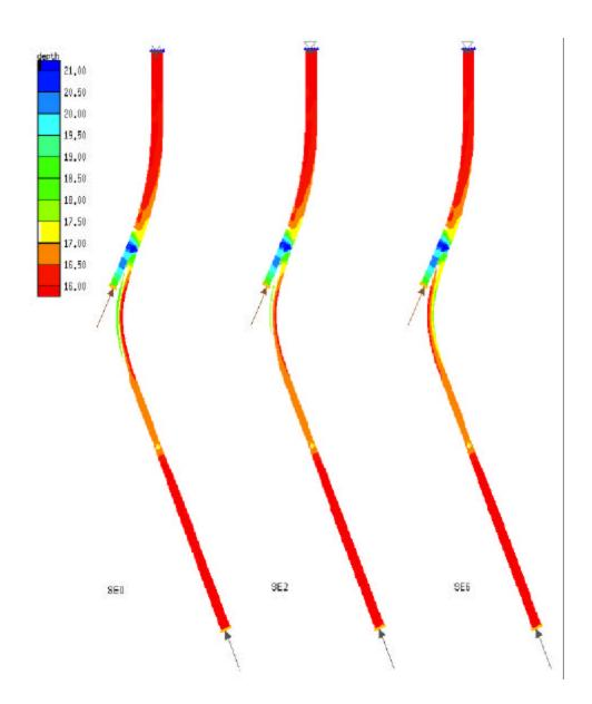
Figure 4.11: Resulting Depths for the Super Elevation Test Cases.
