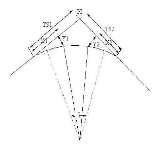
Figure 4.18: Layout of a Circular Curve with Spirals
