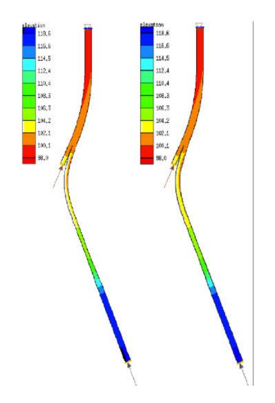
Figure 4.14: Bed Elevations for Channel Widths of 20' (left) and 25' (right).
