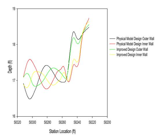
Figure 4.45: Depth Profiles for Physical Model Design and Improved Design.
