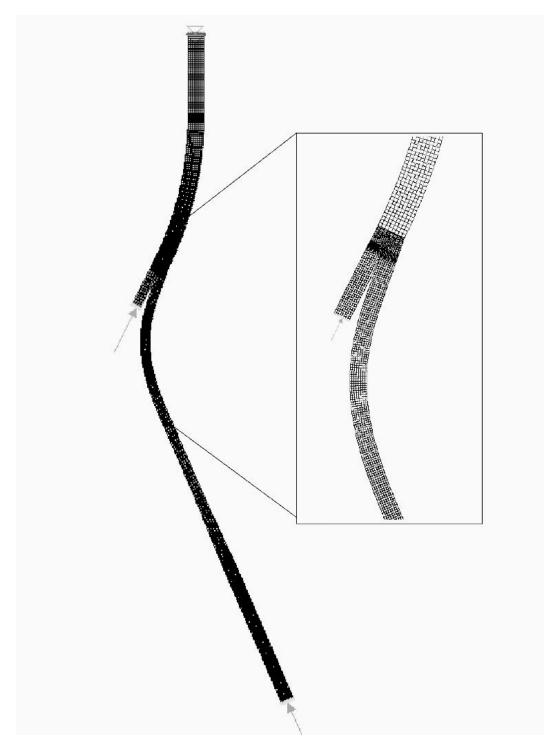
Figure 4.6: The Finite Element Representation and Boundary Conditions.
