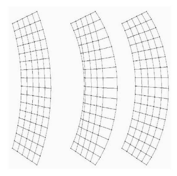
Figure 3.2: Laplacian Smoothing Technique
