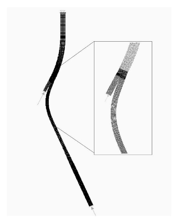
Figure 4.39: Initial Grid for the Radius of Curvature and Super Elevation Problem.
