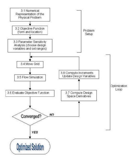
Figure 3.1: Flow Chart of Method for Optimizing High-Velocity Channel
