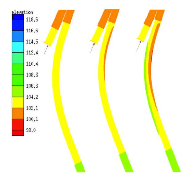
Figure 4.9: Bed Elevations for No(left), 2' (center), and 6' (right) Super Elevation.
