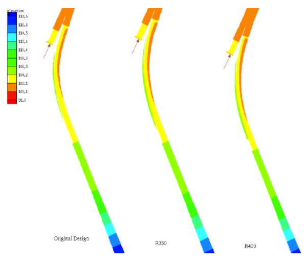
Figure 4.12: Bed Elevations of the Original Curve, 350' Radius, and 400' Radius.
