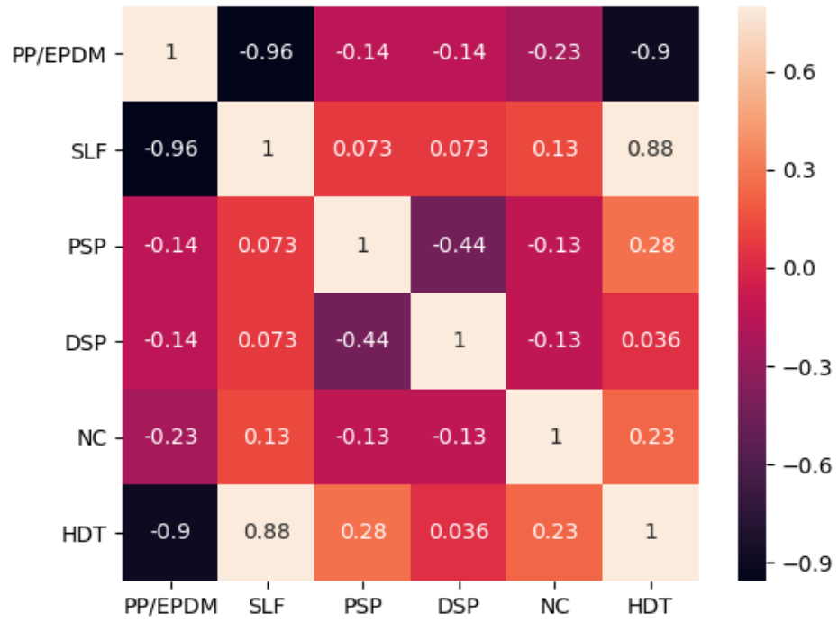
Figure 3.3 Correlation of the features (PP/EPDM, SLF, PSP, DSP and NC) and HDT
