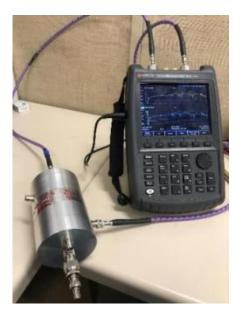
Figure 6.15 Frequency response measurement of D-dot and B-dot.
