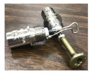
Figure 6.12 Photos of manufactured non-conventional D-dot and B-dot magnetic field sensors
