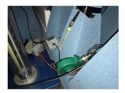
Figure 4.11 Van de Graaff generator and sensors inside the anechoic chamber.
