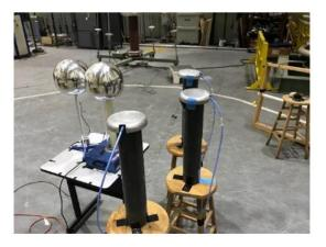
Figure 4.5 Placement of monopole antenna around Van de Graaff generator to establish approximate radiation pattern.
