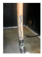
Figure 2.3 Surface discharge propagation along the outer surface of the XLPE cable.
