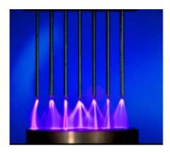
Figure 2.1 Corona discharge in the air [18]
