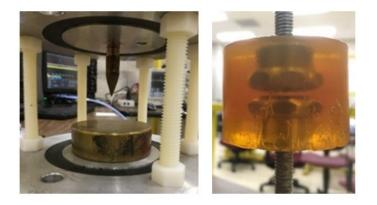
Figure 4.13 Left – corona source using rod-plane conductor configuration; right – cavity discharge using void inside epoxy resin sample.
