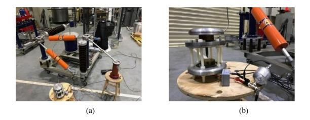
Figure 4.16 Experimental PD test under DC stress. (a) Test setup, (b) Corona test sample.
