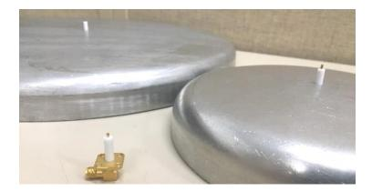
Figure 4.4 Monopole antennas on varying ground planes constructed from SMA connectors.
