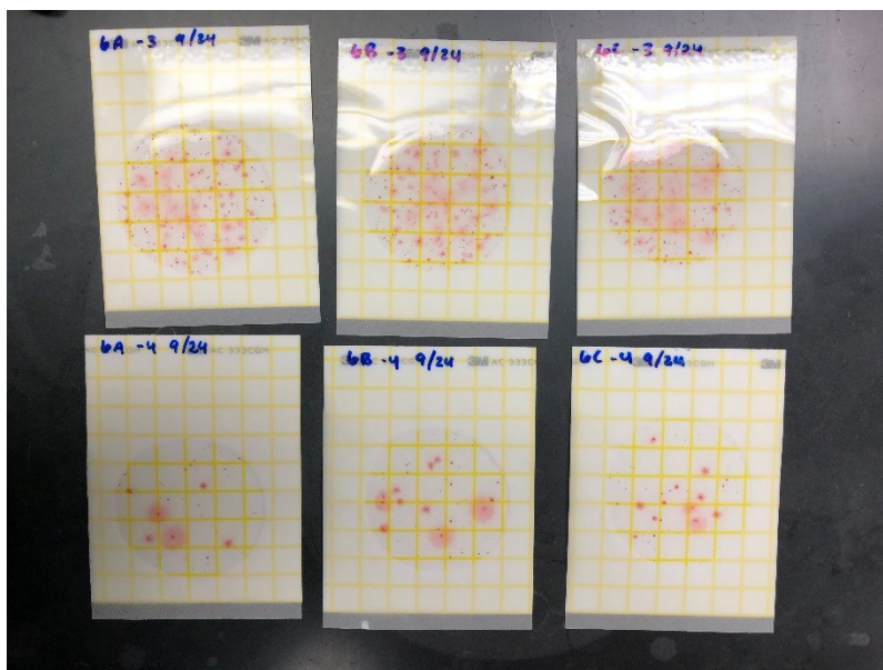
Figure 2.9 The dilution chosen for enumeration showed easily distinguishable colonies Note: The 10^{-4} dilution (bottom) was chosen for bacterial (APC) enumeration because the colonies were more distinguishable than 10^{-3} (top).
