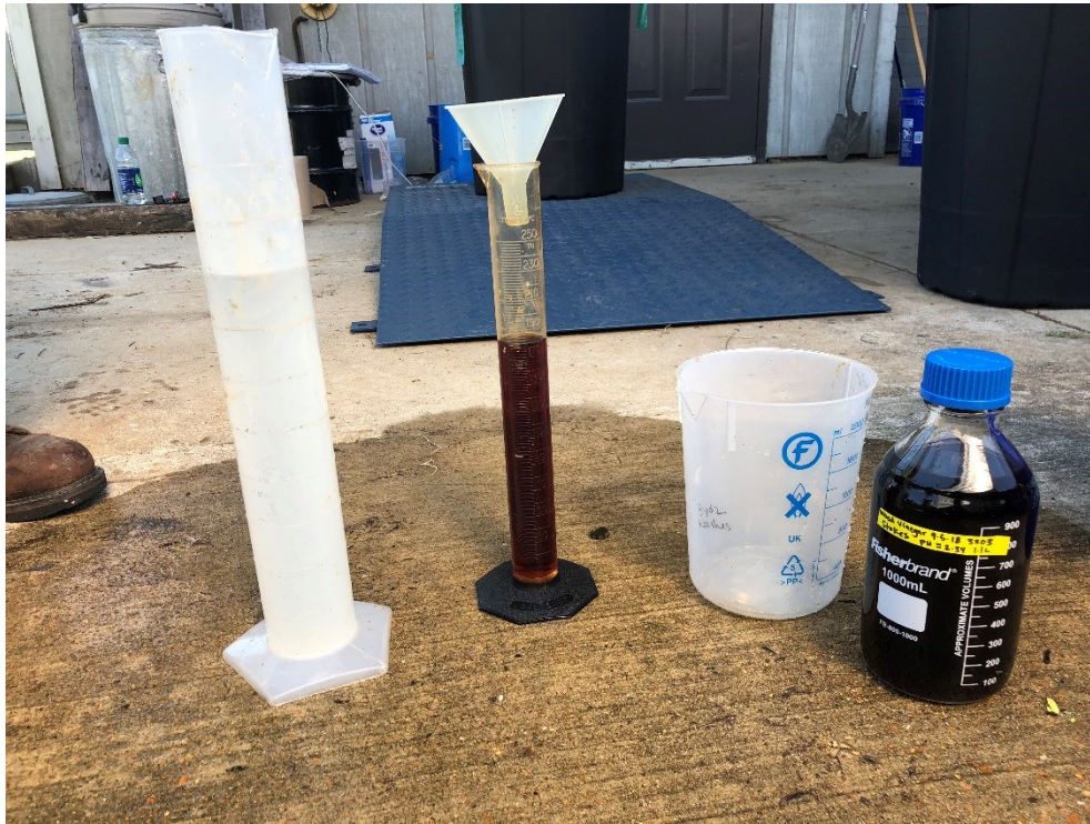
Figure 2.6 Wood vinegar and deionized water were measured to bring the total moisture content of the composts up to 50%.
