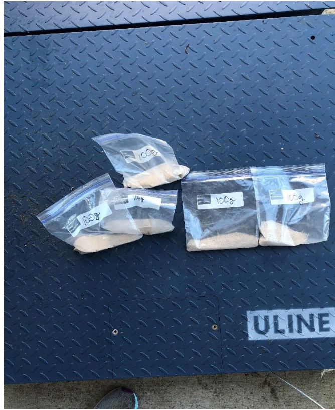
Figure 2.5 Bags containing 0.1 kg of sand were used to improve the accuracy of the scale
