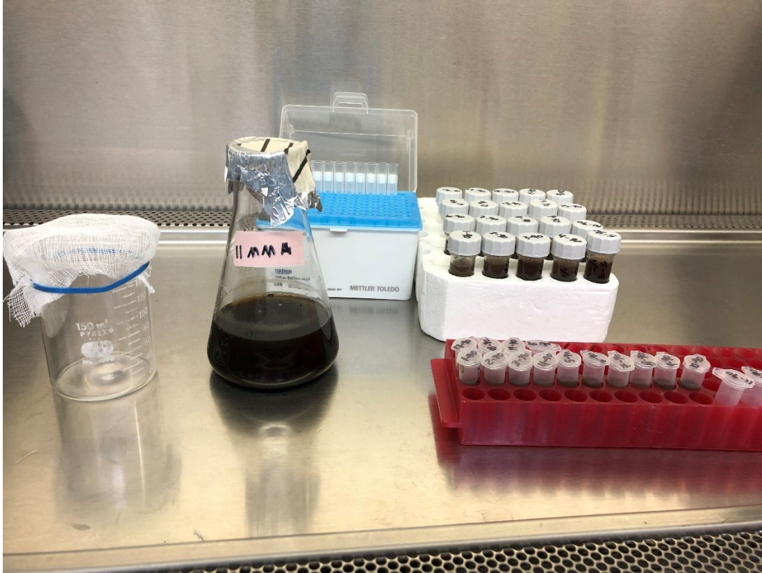
Figure 2.1 Filtration of poultry litter/biochar blends to remove large particulate matter prior to bacterial isolation.
